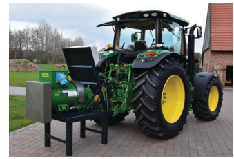
Kemper's 150 kVA emergency power generator, powered by a tractor, ensures that machines with high power consumption can continue agricultural operations in the event of a power outage (source: Kemper)
