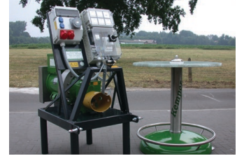
The tools of the Kemper power take-off unit are clearly visible from the tractor: on the left, various plug sockets and the domestic power feed-in; on the right, indicators showing current, voltage and frequencies; below, the generator circuit breaker (source: Kemper)
